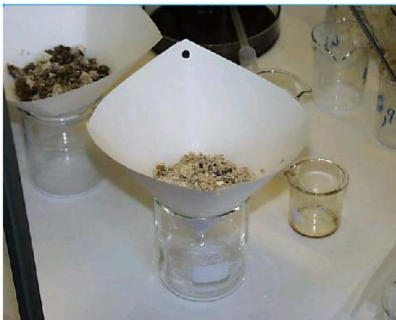
Immediately following each test, the solidified mass was put into a paint filter “drop test” to check for free liquids. After 2-3 hours, each solidified mass was placed on absorbent paper and pressed by hand to check for liquid release. Four of the five masses were completely dry after 3 hours. Phase 4, the bottom phase, had a small wet area indicating that additional drying time was necessary.
