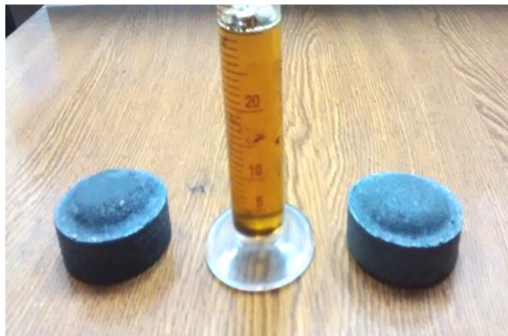
Fig. 12 Samples of Sulfur Composite Waste Form Fig. 13 Solidification Fig. 14 Sodium hydroxide & Volume of Oil Used for Each Form – 30 ml N960 at 3:1 ratio
