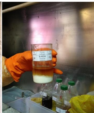
Fig. 12 Samples of Sulfur Composite Waste Form Fig. 13 Solidification Fig. 14 Sodium hydroxide & Volume of Oil Used for Each Form – 30 ml N960 at 3:1 ratio
