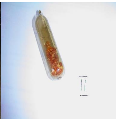
Fig. 11 Irradiation at 770,000 Gray at 30 day's exposure
